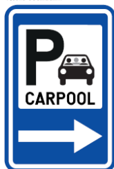
F59 400x600mm quantité 4 Liséré 15mm Txt 45mm Picto 110mm haut P 200mm haut Flèche 300x120mm
